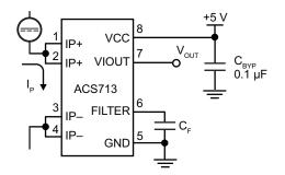
Application 1. The ACS713 outputs an analog signal,  $V_{OUT}$ . that varies linearly with the unidirectional DC primary sampled current,  $I_P$ , within the range specified.  $C_F$  is recommended for noise management, with values that depend on the application.
