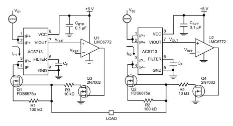
Application 4. Control circuit for MOSFET ORing.
