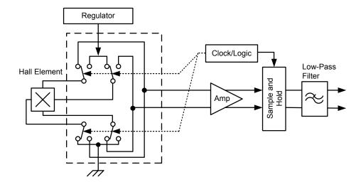
Concept of Chopper Stabilization Technique
